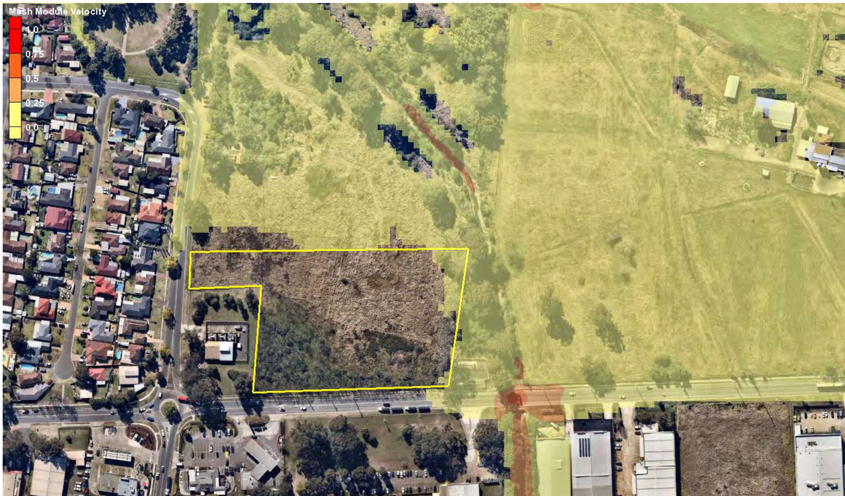
Figure B2.3: 1% AEP Flood Velocity – Post-Development
